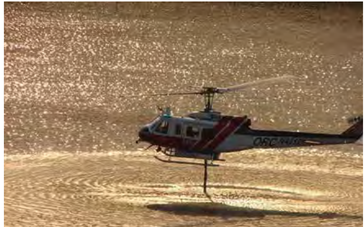
OCFA helicopter uses a snorkel to refill its water tank.
